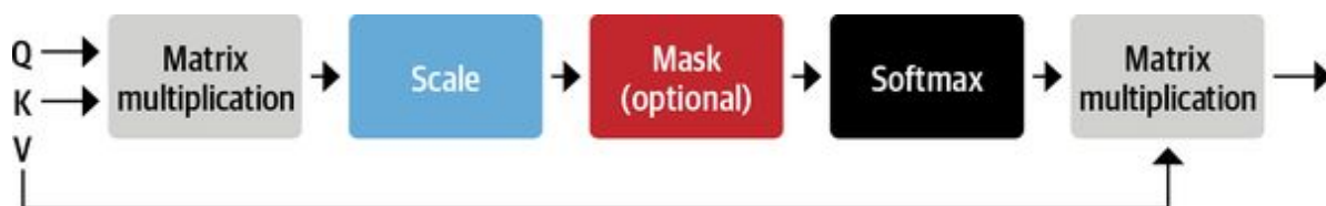
Figure 3-4. Operations in scaled dot-product attention
