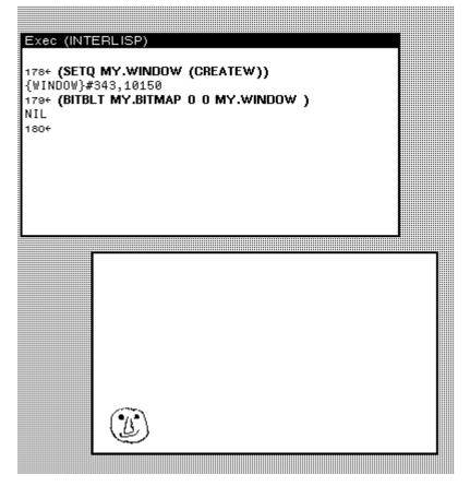
Figure 14-5. BITBLTing a Bitmap onto a Window
