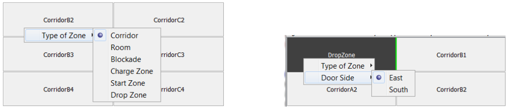
(a) the drop down menu generated when a zone is right clicked (b) the drop down menu generated when a room is right clicked
